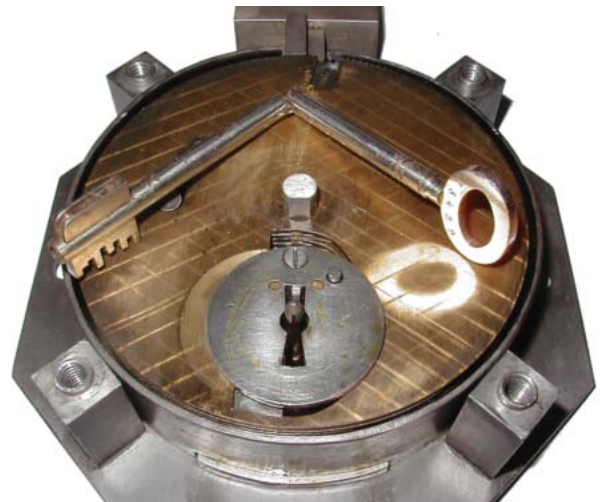
Arnhem's Lammellenschloss with its giant (110mm diameter) circular disc like levers, all entirely springless.
