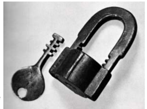
Polhem's Padlock, entirely spring-less and eminently suitable for harsh environments but also greatly improving security at the time.
