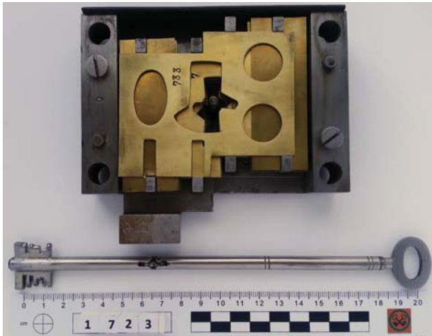
Arnhem's springless 'Colosseum' lock, the levers first move horizontally and then vertically.
